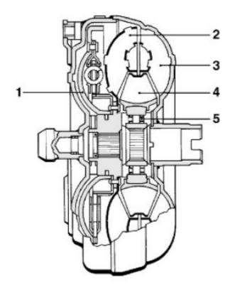
Figure 9.3: Hydrodynamic converter with lockup clutch
