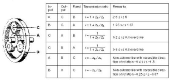
Basic equation for planetary-gear sets:  $n_{\rm A} + (Z_{\rm B}/Z_{\rm A}) \cdot n_{\rm B} - (I + Z_{\rm B}/Z_{\rm A}) \cdot n_{\rm C} = 0$
