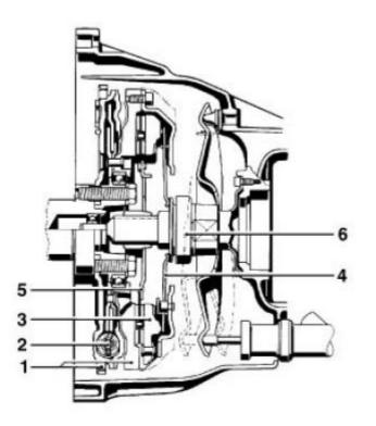
Figure 9.1: Clutch with dual-mass flywheel
